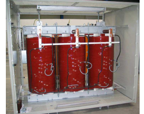
15kV, 1,200kVA, compact design transformer with rectifier, for power supply of tramway traction system;.
