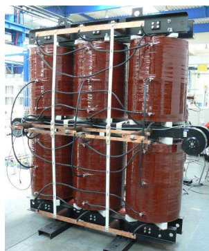
24-pulse transformer for feeding of frequency converter 50/60Hz with power of 1,600 kVA and system voltage of 15kV;
